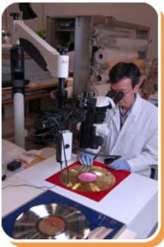
A conservator uses a stereomicroscope to carefully remove residues of corrosion on a gold disc.
